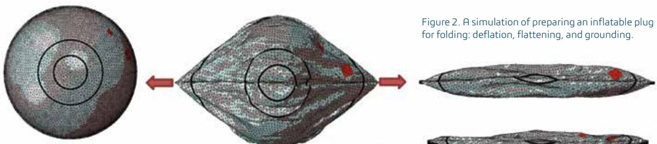
Figure 2. A simulation of preparing an inflatable plug for folding: deflation, flattening, and grounding.
