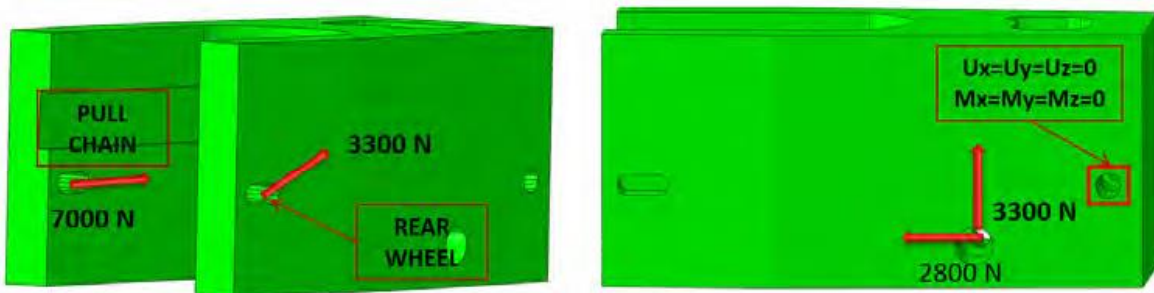
Figure 5. Load Case 1: Service loads acting on swing arm due to passenger load.
